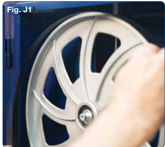
2. Replacing the blade is simply the same procedure in reverse, understanding that the bearing guides may need adjustment to accommodate the new blade. **Remember to re-lock everything and adjust your tension and guides systems before use!**
