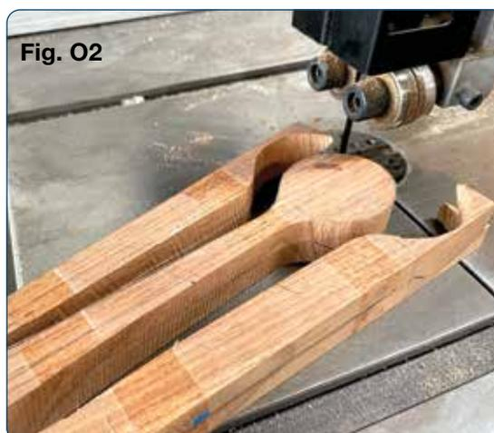
5. If you find yourself in a difficult cut where you cannot continue, don't force the work through but switch off your saw, wait for it to stop and manually removing or reverse the board from the cut.
